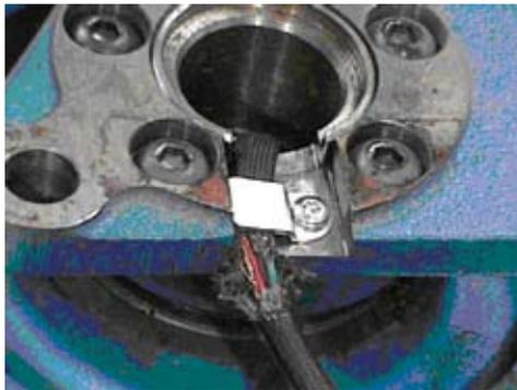
Figure 1 Frayed wire
