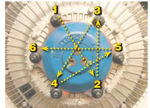
Figure 3 Torque sequence
